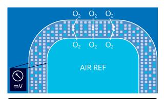
ZIRCONIUM OXIDE SENSOR SCHEMATIC Figure 7. While this sensor gives quick readings, it must be used in applications containing hydrocarbon levels that are greatly below the oxygen concentration.
