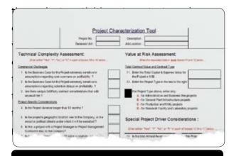
SAMPLE CHARACTERIZATION TOOL Figure 2. Tool uses yes/no answers for most questions and pre-determined weights to place project into a particular class.
