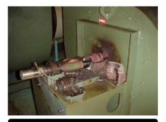
BEARING LUBRICATION Figure 3. Lack of proper bearing lubrication compromised this fan's performance.
