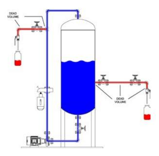
DEAD VOLUME Figure 3. Dead volume in a sample station can lead to plugging.
