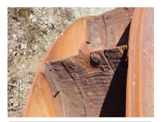
FAN WEAR Figure 4. Depending on the application, ask your van vendor for suggestions for proper protection from wear.
