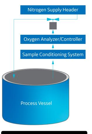
SCHEMATIC FOR TANK INERTING WITH O2 ANALYZER Figure 2. Adding an oxygen measurement will indicate potentially dangerous conditions.
