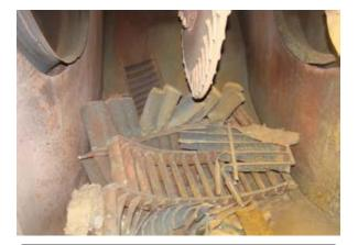
WHEEL FAILURE Figure 2. Addressing past performance issues such as this wheel failure can help you properly select a new fan and avoid such issues from repeating.
