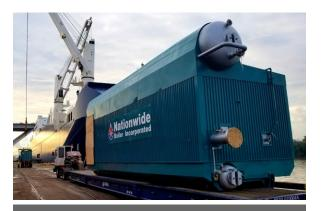
WATER TUBE BOILER Figure 4. This 200,000-lb/hr package water tube boiler is ready for a long-term rental overseas.
