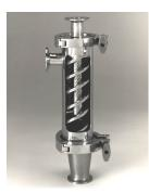
Sanitary Heater is an excellent choice for cooking slurries with bite-sized pieces such as salsas and sauces. It was the first DSI heater to achieve setpoint temperature on demand with a non-shearing action. The unique, low velocity, multiple orifice steam injector and helical flights ensure proper blending
