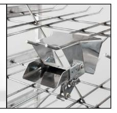
This has led to the development of roll-in type batch washers that are provided with specialized wash racks for buckets, feeder pans and chutes. Typically, batch washers feature a recirculating detergent wash tank and a separate fresh water, sanitizing rinse tank. In the case of Douglas Scale Parts Washers, cycles are selected from a short, medium or long sequence (4, 6 or 8 minutes) depending on soil conditions.
