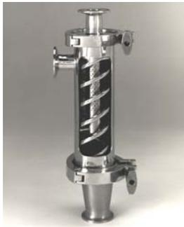
for cooking slurries with bite-sized pieces such as salsas and stews. It was the first DSI heater to achieve set-point temperature on demand with a non-shearing action. The unique, low velocity, multiple orifice steam injector and helical flights ensure proper blending of steam and
