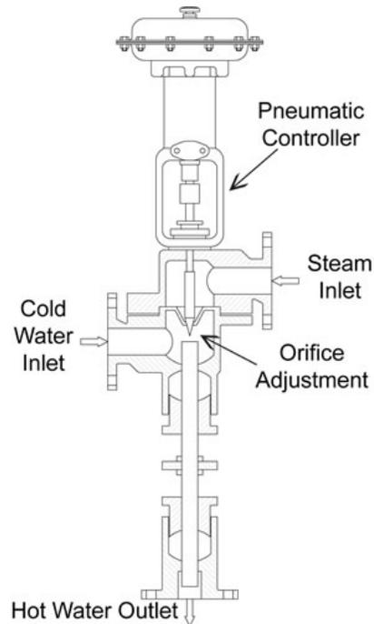
**Figure 3. Venturi Steam Injector**
