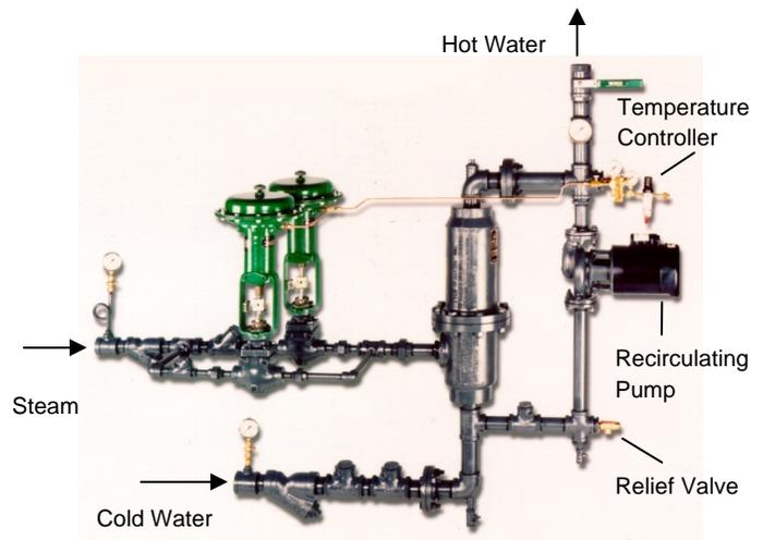
**Figure 4. Dual Modulating Steam Injection Control System**
