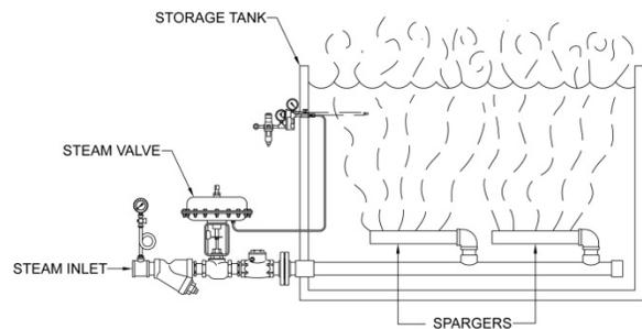
**Figure 1. Spargers heat water in an open tank by bubbling steam up through it.**
