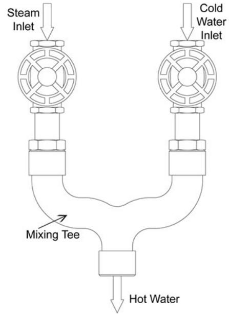
**Figure 2. Manual Mixing Tee**
